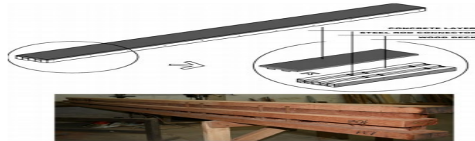
Figure. 3 Wood–concrete beam and horizontal shear connection detail [10]
