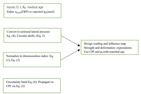
Note.  $p_0$ , normalization to CPI using Eqs. (1)–(3), and propagation of measurement and model scatter to an uncertainty band using Eq. (6) [1,2,3,6,7].
